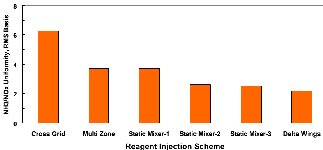
Figure 5. NH 3 /NO Uniformity (RMS Basis): Various Reagent Injection Schemes
